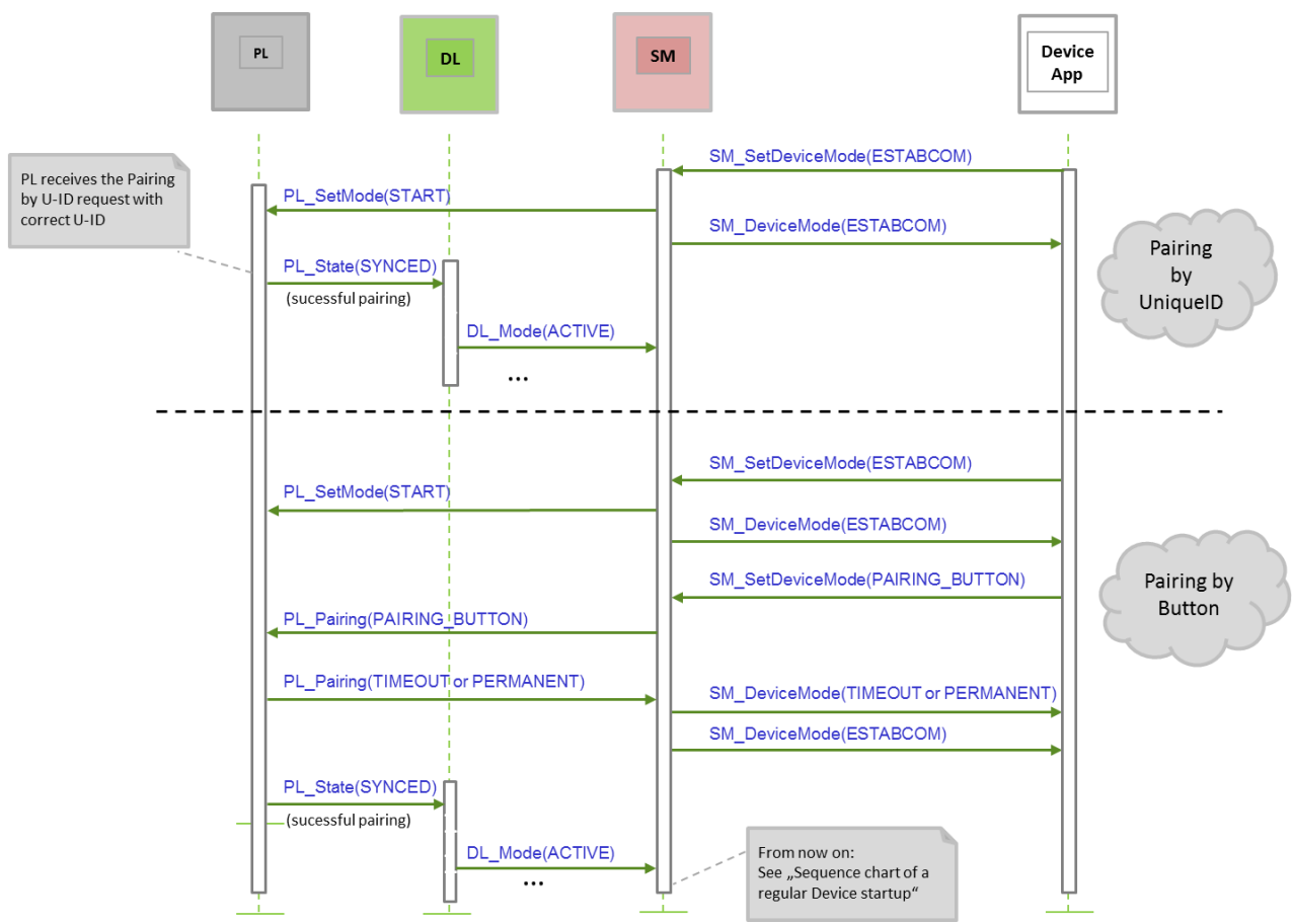
Figure 105 Sequence chart of a Device pairing
